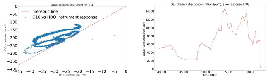
Large deviations from the meteoric line in the gas phase instrument illustrates two issues. 1) Lack of heating of instrument flow lines combined with 2) a slow flow rate makes concentration events much more of an issue for the gas phase instruments. These issues will be addressed in IMPACTS 2022 to make this data reliable.
